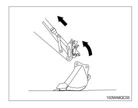
(9) To lock the quick coupler, release the quick coupler button on the right joystick lever.
